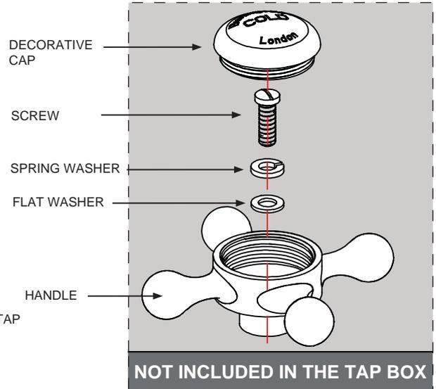
Note: To ensure the Kensington lever tap head faces in the correct forward position once installed, you may need to tighten the cartridge into the tap body a notch with a monkey spanner and then re-attach the tap head.
