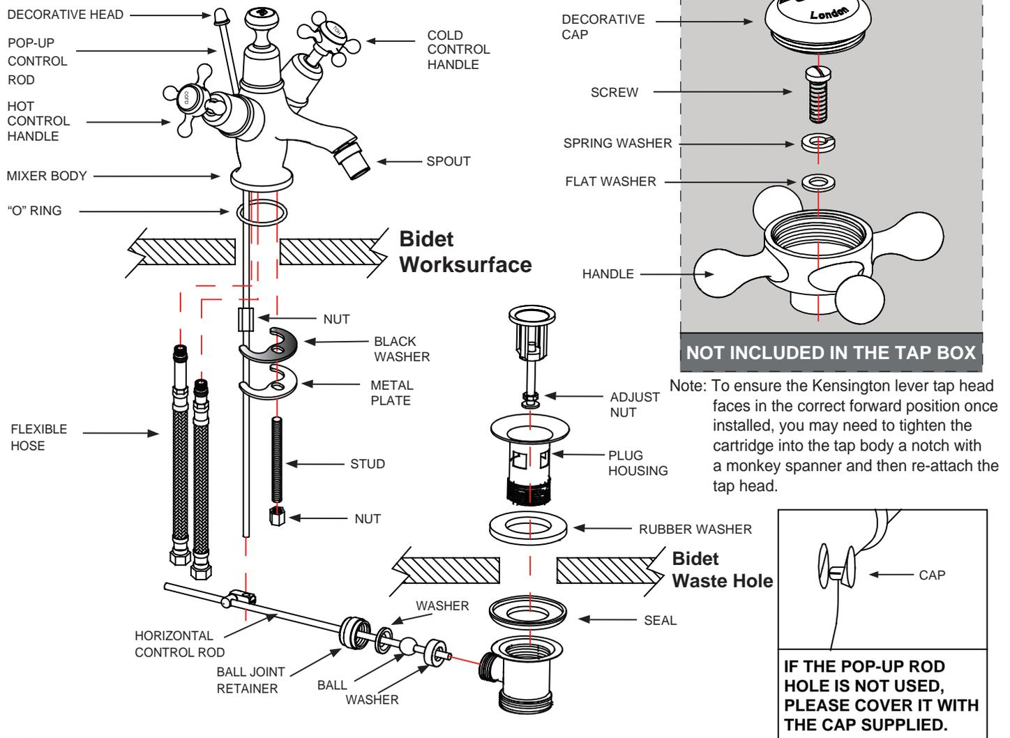
1. Fit the "O" ring into the groove on the underside of the mixer body.
