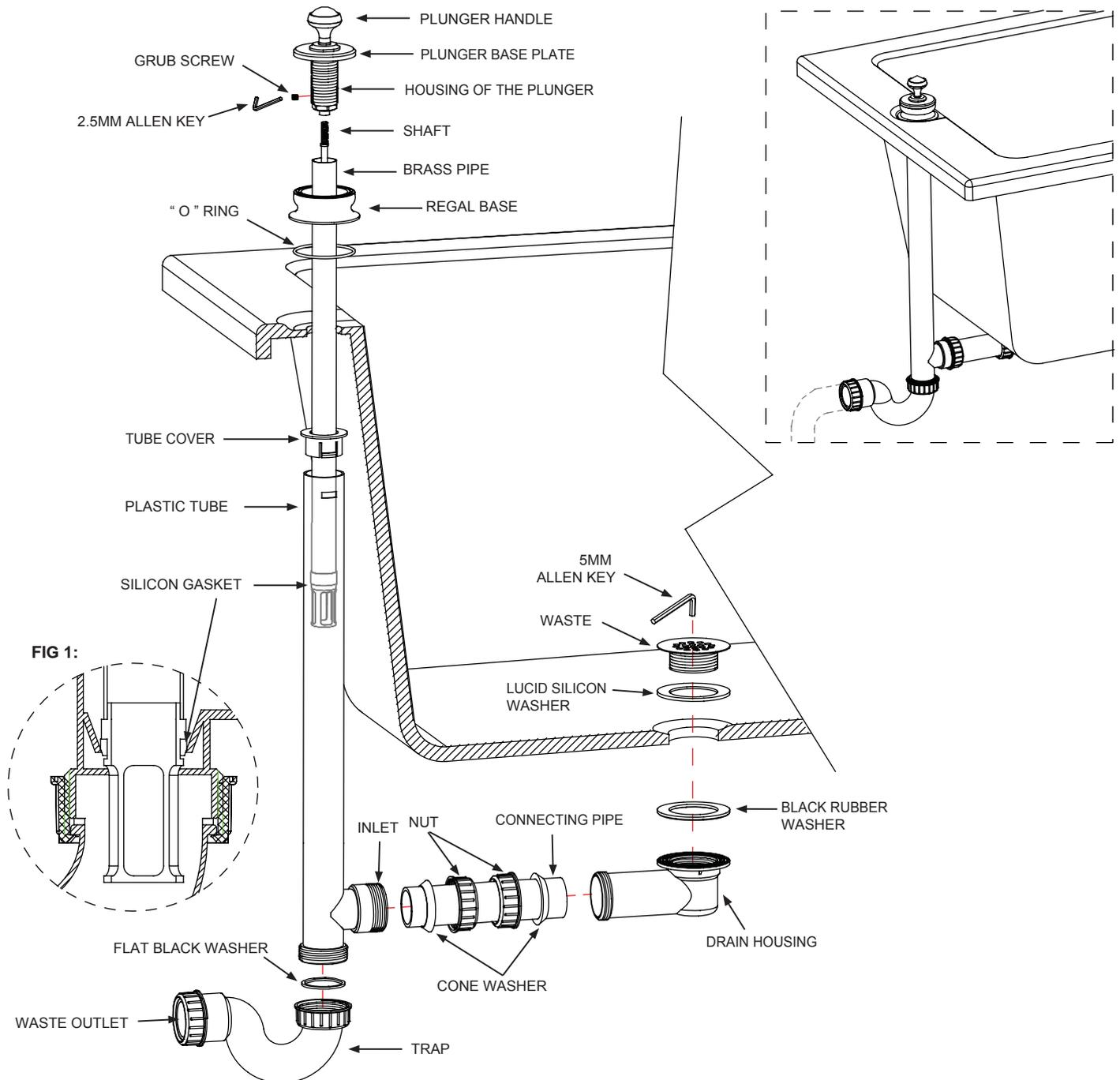
1. Remove the tube cover from the plastic tube, and take out the brass pipe.
